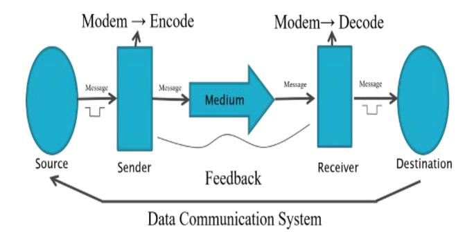
**Source:** The device from which data is sent. Example- Computer, Telephone, Mobile Phone etc.
