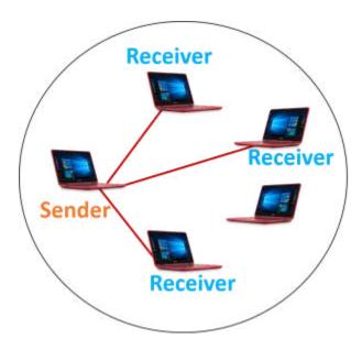
This is useful when a device in one network wants to transfer packet stream to the selected devices over the other network.
