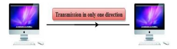
The radio station is a simplex channel as it transmits the signal to the listeners but never allows them to transmit back. Keyboard and Monitor are the examples of the simplex mode as a keyboard can only accept the data from the user and monitor can only be used to display the data on the screen.
