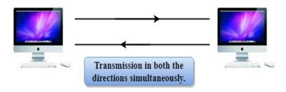
The most common example of the full-duplex mode is a telephone network. When two people are communicating with each other by a telephone line, both can talk and listen at the same time.
