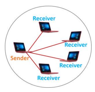
This is useful when a device in one network wants to transfer packet stream to all the devices over the other network.
