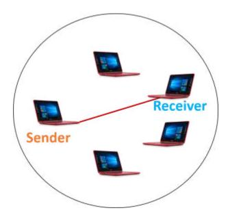
For example, a device having IP address 10.1.2.0 in a network wants to send the traffic stream(data packets) to the device with IP address 20.12.4.2 in the other network, then unicast comes into picture. This is the most common form of data transfer over the networks. The devices such as switches use unicast mode of transmission.
